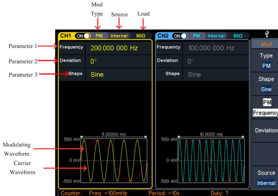
Figure 5-13: Phase modulation user interface
