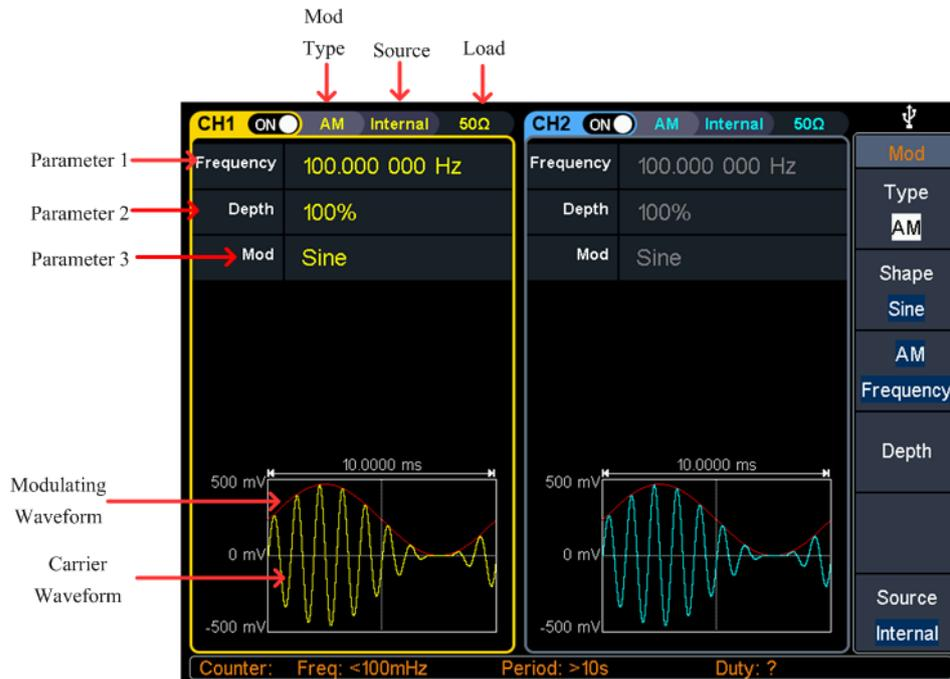
Figure 5-11: Amplitude modulation user interface
