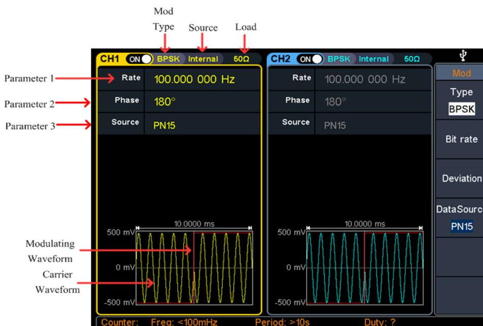
Figure 5-20 Binary phase shift keying user interface
