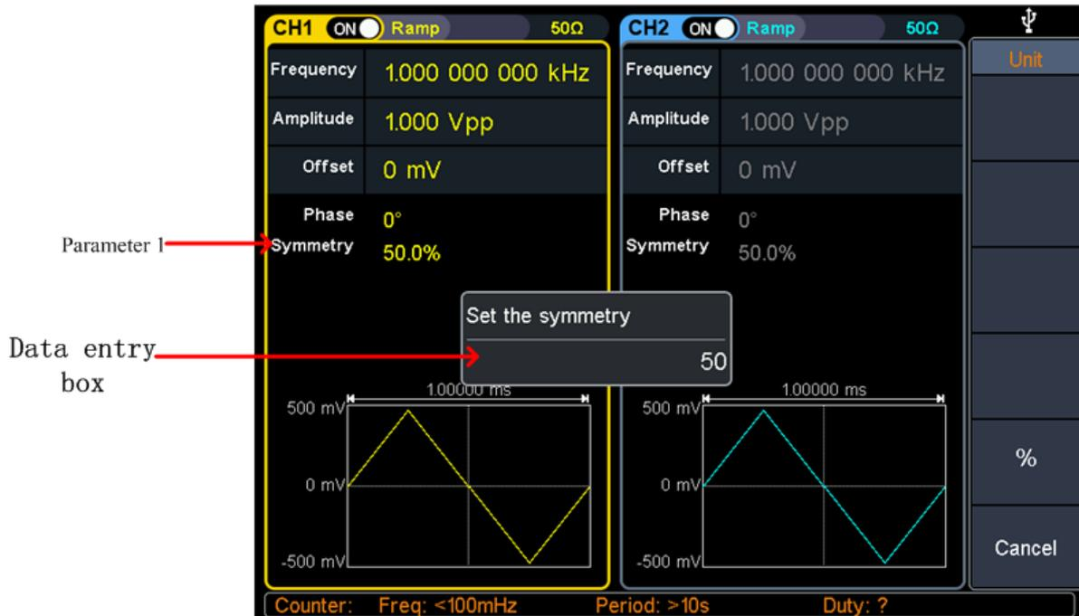
Figure 5-5: Set the symmetry of ramp wave
