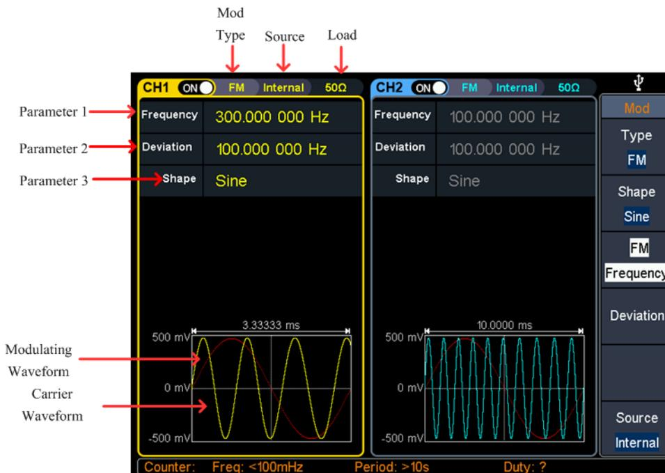
Figure 5-12: frequency modulation user interface
