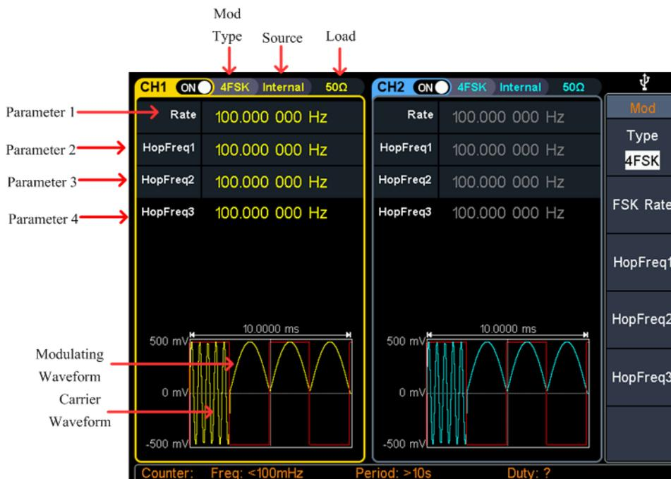
Figure 5-19 Quaternary frequency shift keying user interface
