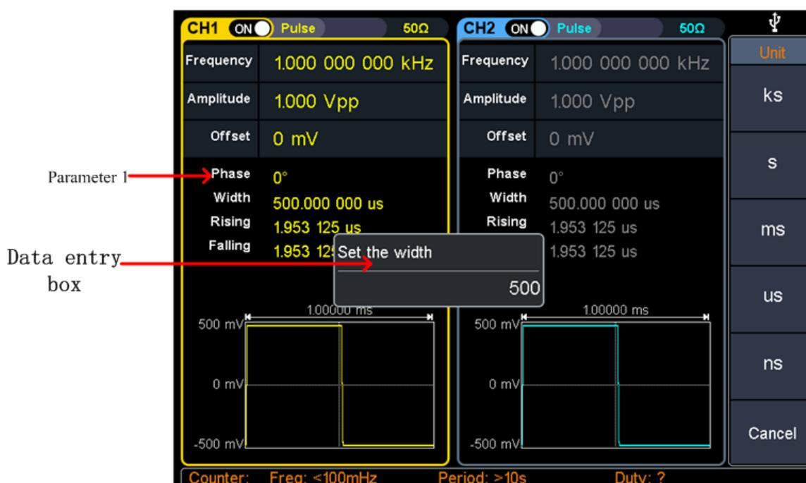
Figure 5-7: Set the pulse width
