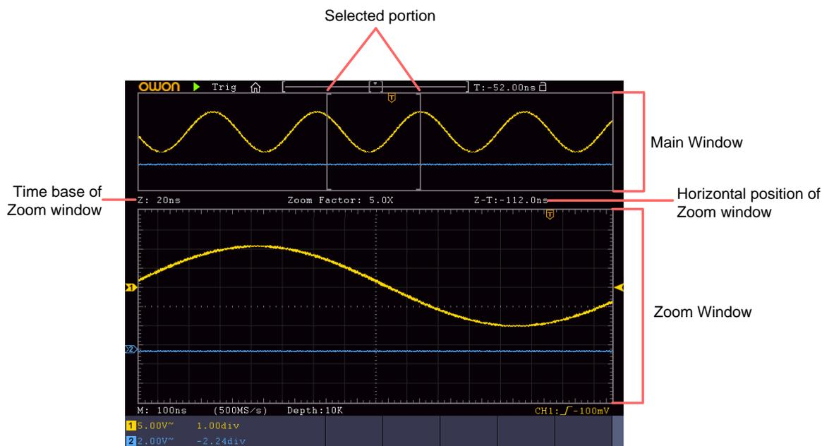
In normal mode, the **Horizontal Position** and **Horizontal Scale** knobs are used to adjust the horizontal position and time base of the Main window.
