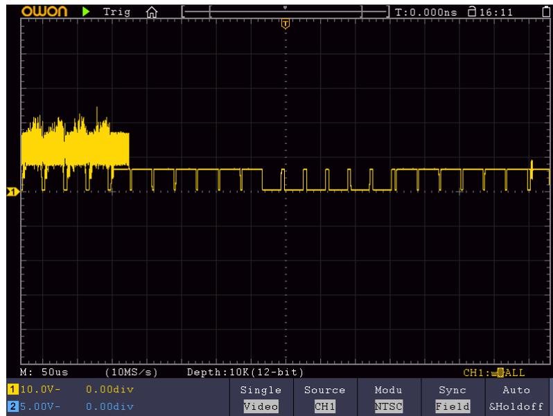
Figure 9-7 Waveform Captured from Video Field Trigger
