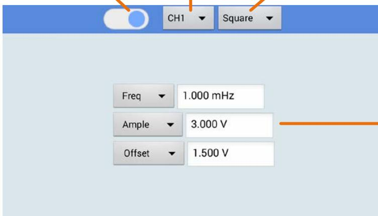
Set the parameters of current waveform
