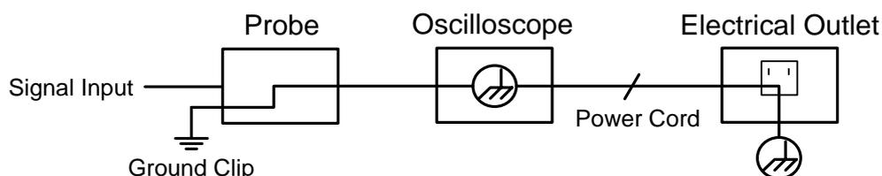
**The diagram of the ground wire connection when the battery-powered oscilloscope is connected to the AC-powered PC through the ports:**
