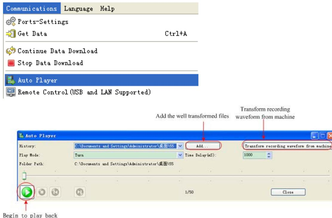
Figure 4-19: Play back waveform by software
