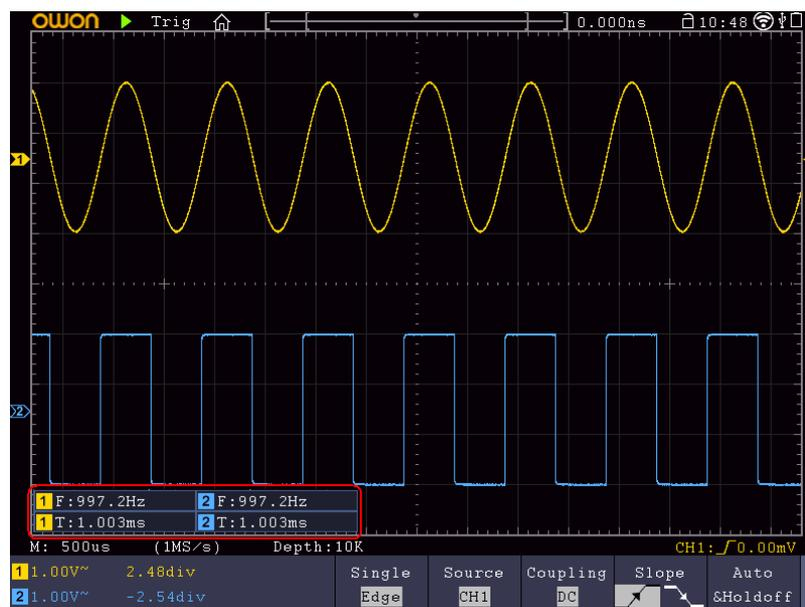
Figure 4-20 Automatic measurement
