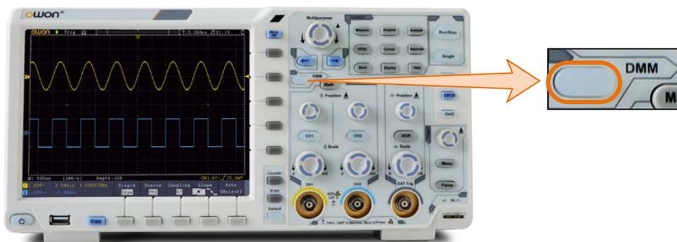
Figure 6-2 Multimeter Button
