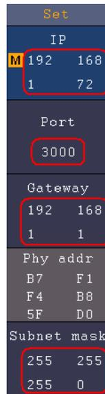
Figure 7-7 Set the network parameters of the oscilloscope
