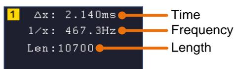
**Note:** If "Out Of Limits" appears in the information or a message "Waveform points beyond the limit." appears on the screen, that means the length of the cloned waveform exceeds the limit. When the source is CH1 or CH2, the maximum length is 2M; When the source is CH1&CH2, the maximum length is 1M. Push the **Acquire** button, select **Length** in the bottom menu, and set the record length to a smaller value.
