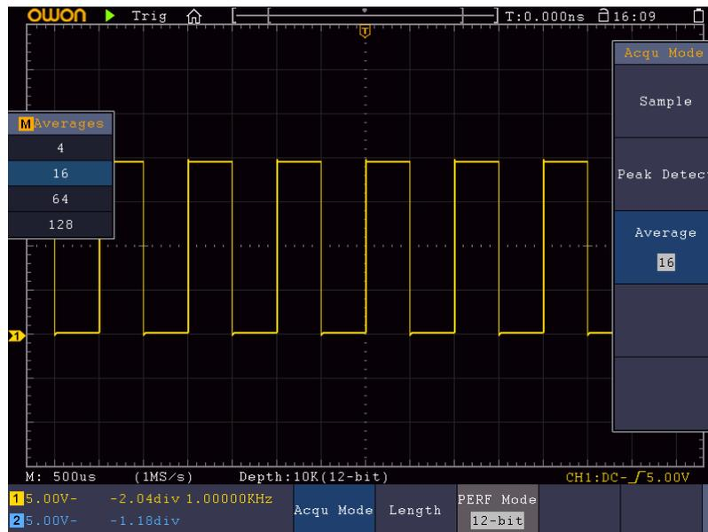
Figure 9-5 Reduce Noise level by using Average function
