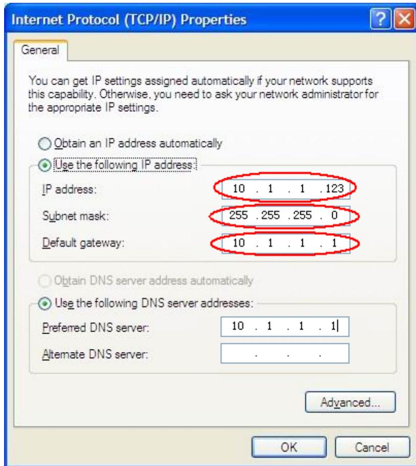
Figure 7-9 Set the network parameters of the computer
