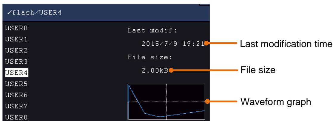
If a USB device is connected, and you want to save the waveform to it, select **Memory** in the right menu as **USB**. The instrument lists a directory of the folders and files on the USB memory device. Select a folder or file using the **M** knob to scroll up
