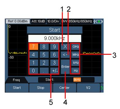
Figure 5-2 Numeric keypad interface
