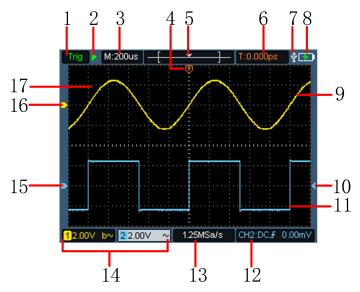
Figure 3-3:Oscilloscope Interface
