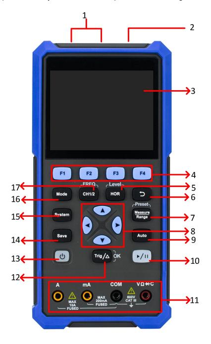
Figure 3-1:Front Panel of the Oscilloscope
