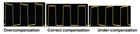
Figure 3-5: Display Waveform of Probe Compensation
