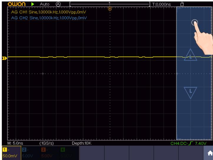
When the **L** icon appears, in the full screen, swipe up/down to control the trigger level of the source in the trigger menu.
