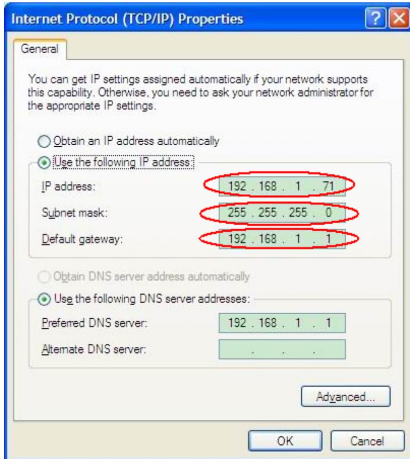
Figure 6-5 Set the network parameters of the computer
