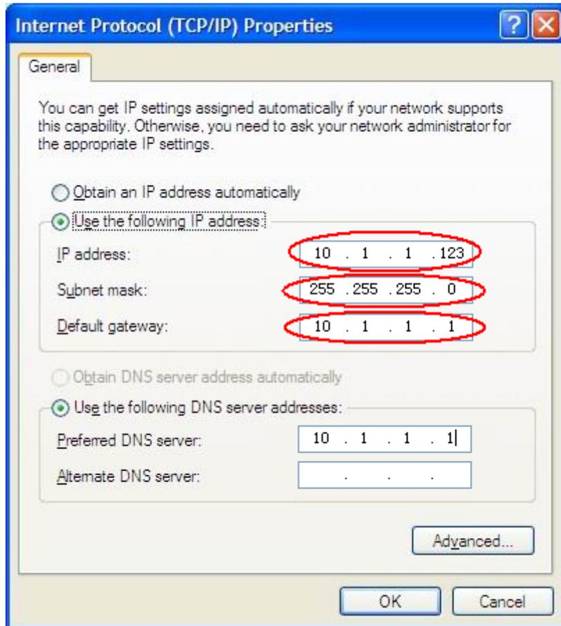
Figure 6-9 Set the network parameters of the computer
