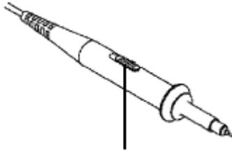
Figure 3-8 Attenuation Switch
