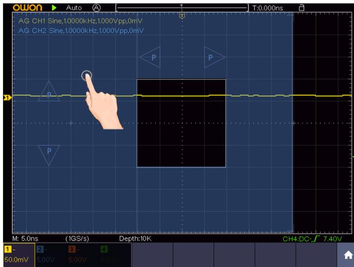
When the P icon appears, in the full screen, swipe left/right to control the horizontal position, swipe up/down to control the vertical position of the selected channel.
