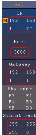
Figure 6-7 Set the network parameters of the oscilloscope
