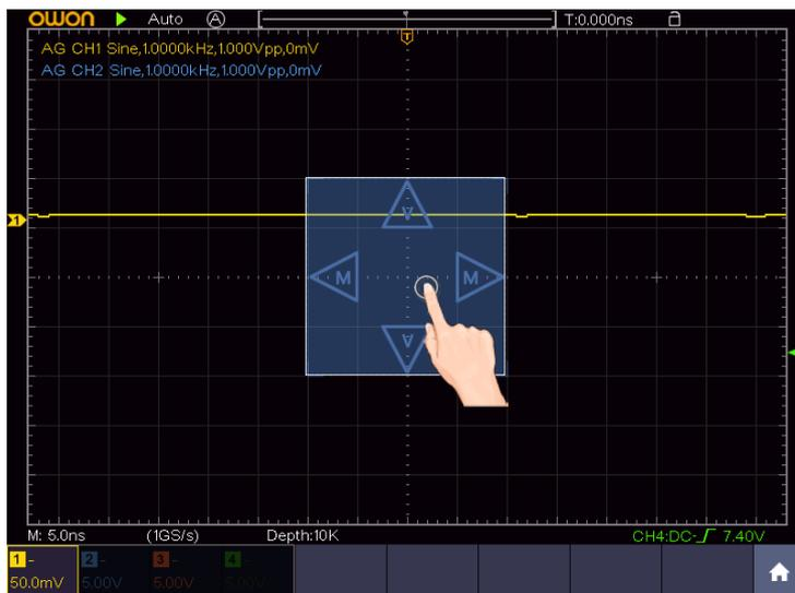
When the M and V icons appear, in the full screen, swipe left/right to change the time base, swipe up/down to change the voltage division of the selected channel. Click the icons to fine-tune, long-press to adjust continuously.
