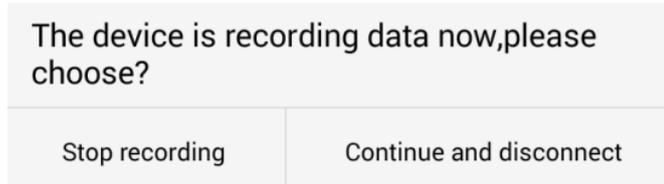
Select **Stop recording**, the recording process will be interrupted. The Android device will connect with the multimeter to read data.
