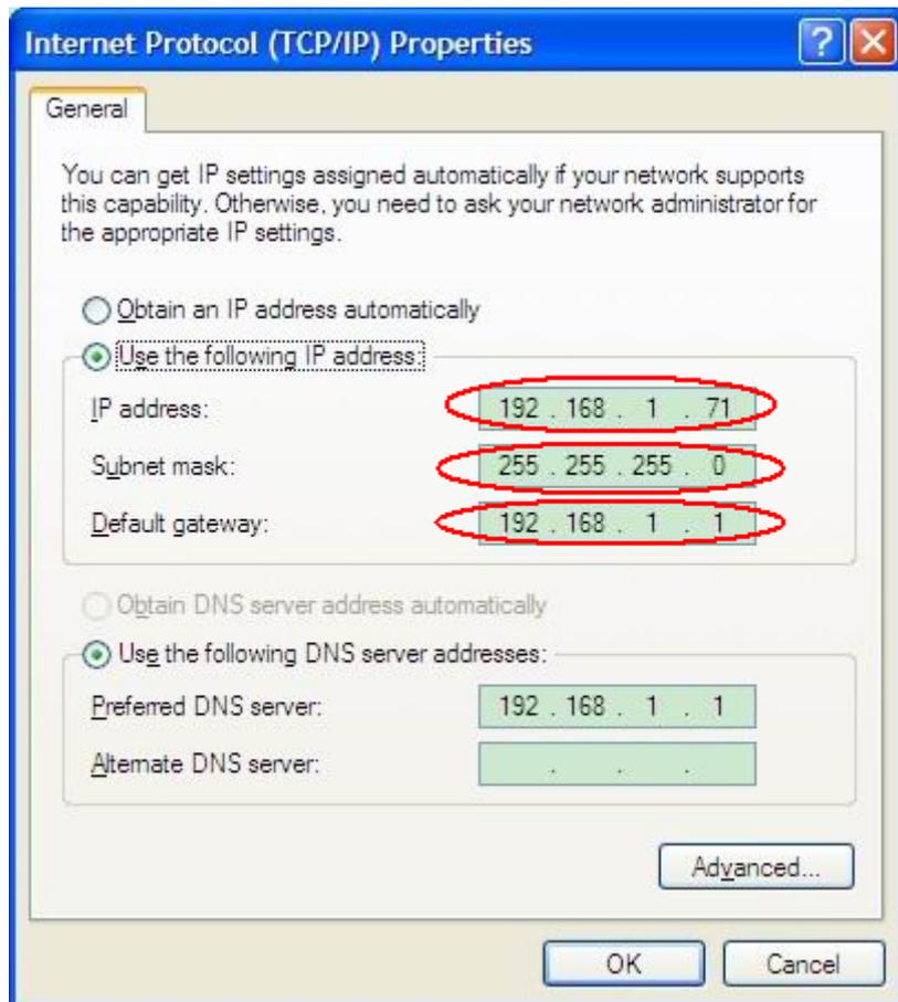
Figure 4-5 Set the network parameters of the computer
