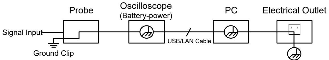
**It is not allowed to measure AC power when the oscilloscope is AC powered, or when the battery-powered oscilloscope is connected to the AC-powered PC through the ports.**
