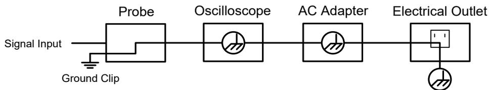
**The diagram of the ground wire connection when the battery-powered oscilloscope is connected to the AC-powered PC through the ports:**
