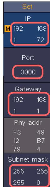
Figure 4-7 Set the network parameters of the oscilloscope
