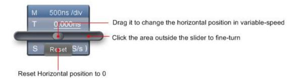
to reset the horizontal position of the signal, via moving the slider leftwards, or rightwards - the farther slider from the center of control bar, the faster the horizontal position changes; or through dragging the red pointer to reset the horizontal position of the signal (as item 3 goes under VII. Operation Interface of PC Software).
