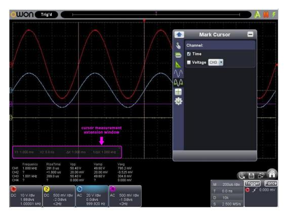
**voltage cursor measurement:** Check "Voltage" option, from the horizontal direction of main display area, two lines in light color appears, indicating Cursor 1 and Cursor 2.
