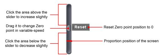
to reset zero point position will change the vertical position of the signal, via moving the slider upwards, or downwards - the farther slider from the center of control bar, the faster the vertical position changes.
