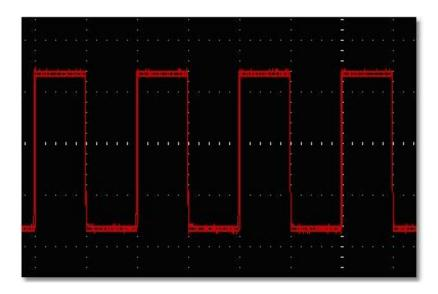
Following illustration is signal output under Average mode, with average number set in 16, from here, the interrupting signal noise been reduced to certain degree,
