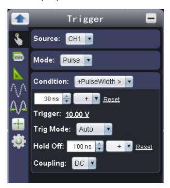
The **Trigger** option here indicate single trigger, it is the one to use one trigger signal to capture data from two channels, simultaneously, the operation steps -
