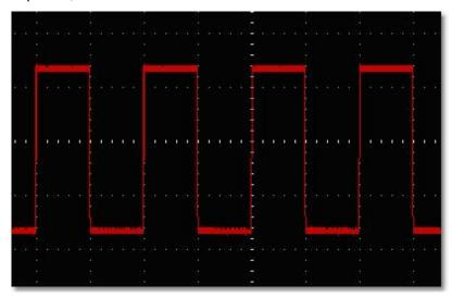
Following illustration is signal output under Peak Detect mode, the interrupting signal noise been captured in details,
