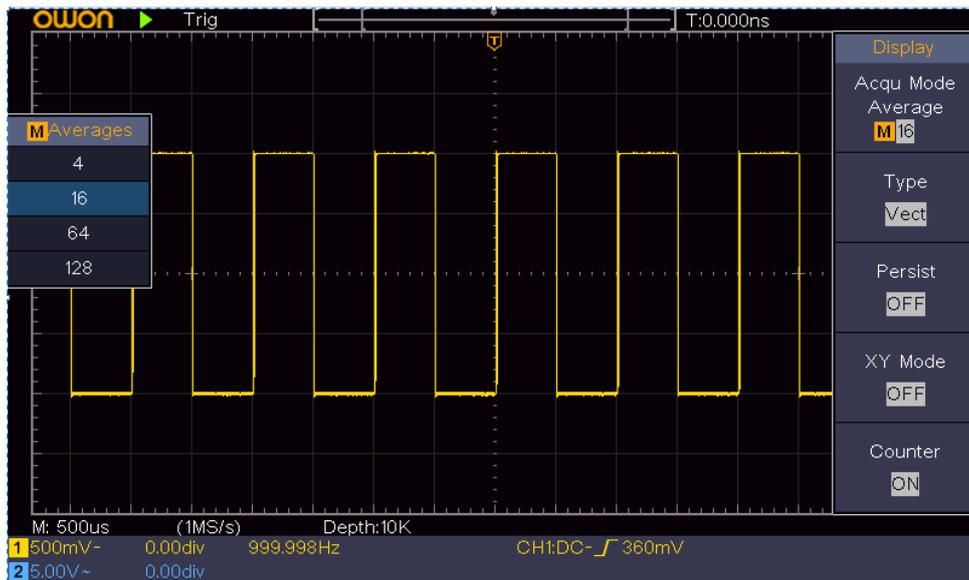
Figure 6-5 Reduce Noise level by using Average function
