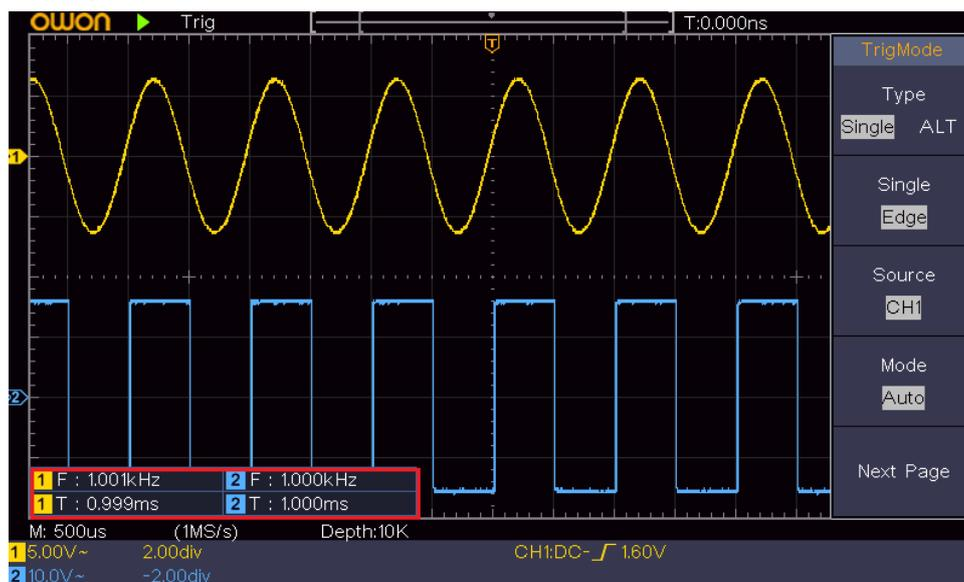
Figure 4-12 Automatic measurement
