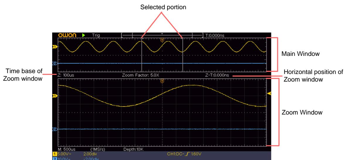
In normal mode, the **Horizontal Position** and **Horizontal Scale** knobs are used to adjust the horizontal position and time base of the Main window.
