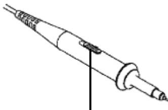
Figure 3-8 Attenuation Switch
