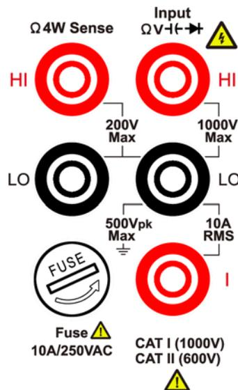
The user-replaceable 10 A current-protection fuse is on the front panel. To maintain protection, replace fuse only with fuse of the specified type and rating. About the specified type and rating of the fuse, please refer to "7 Current Terminal Fuse" in "Front Panel Overview" on page 6.
