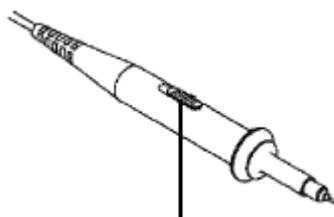
Figure 3-9 Attenuation Switch
