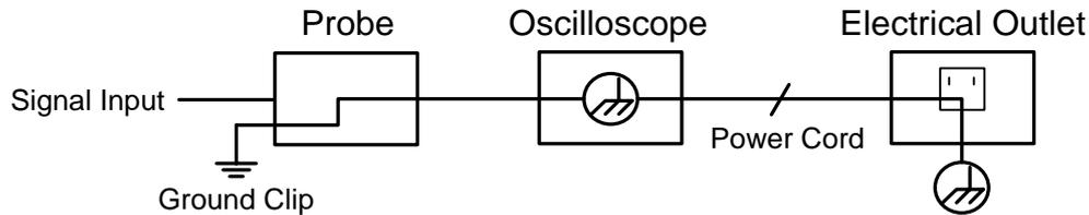
It is not allowed to measure AC power when the oscilloscope is AC powered.
