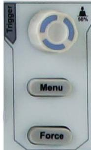
Figure 3-13 Trigger Control Zone
