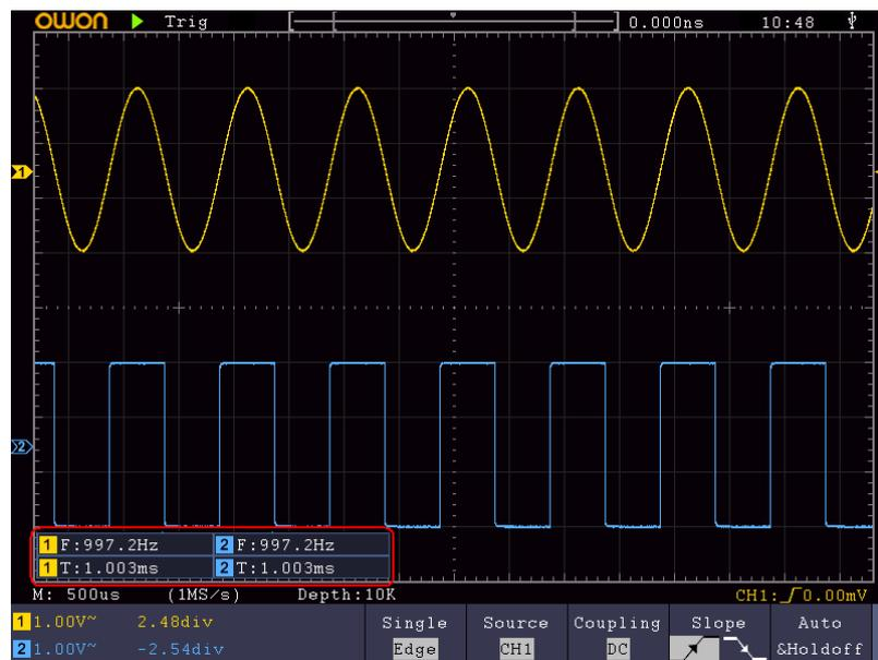
Figure 4-13 Automatic measurement
