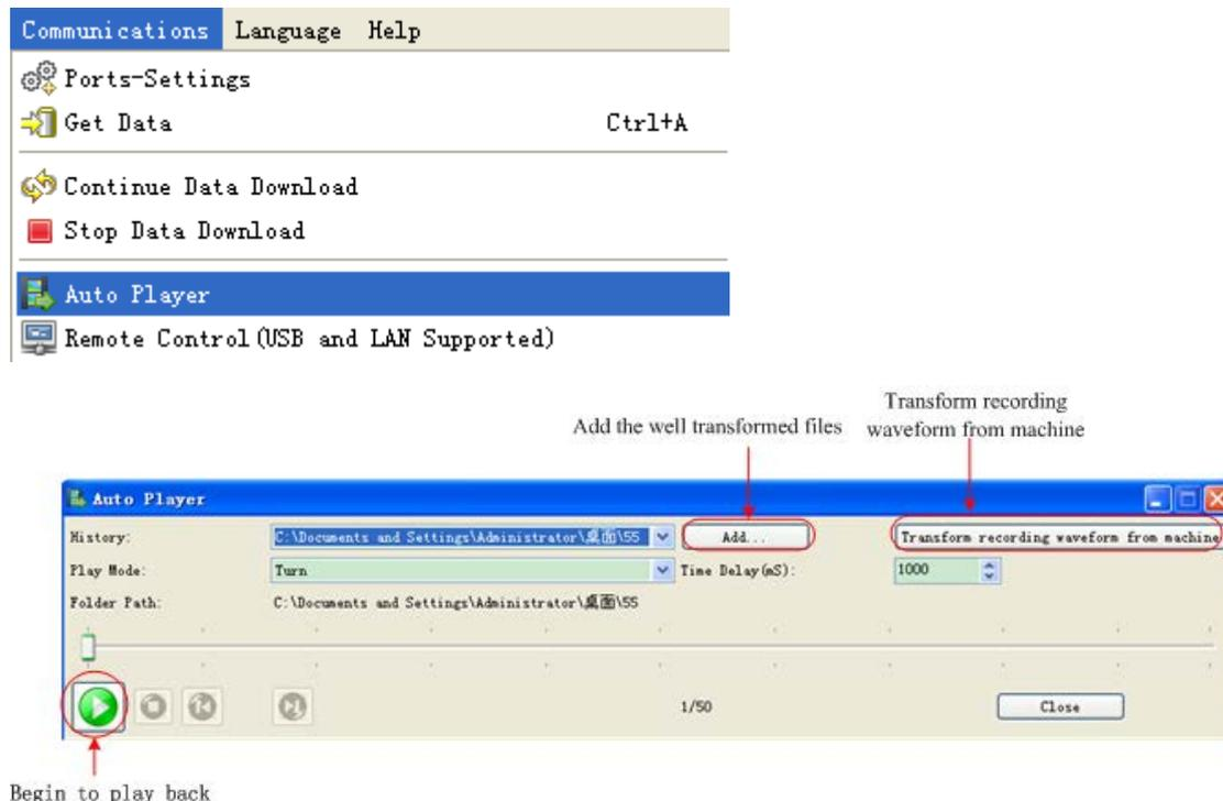
Figure 4-12: Play back waveform by software
