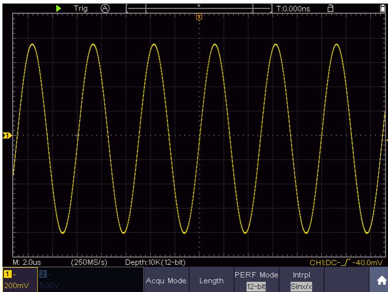
Figure 4-4 Sine(x)/x interpolation
