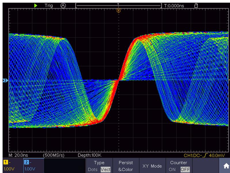
Figure 4-6 The color temperature function is on
