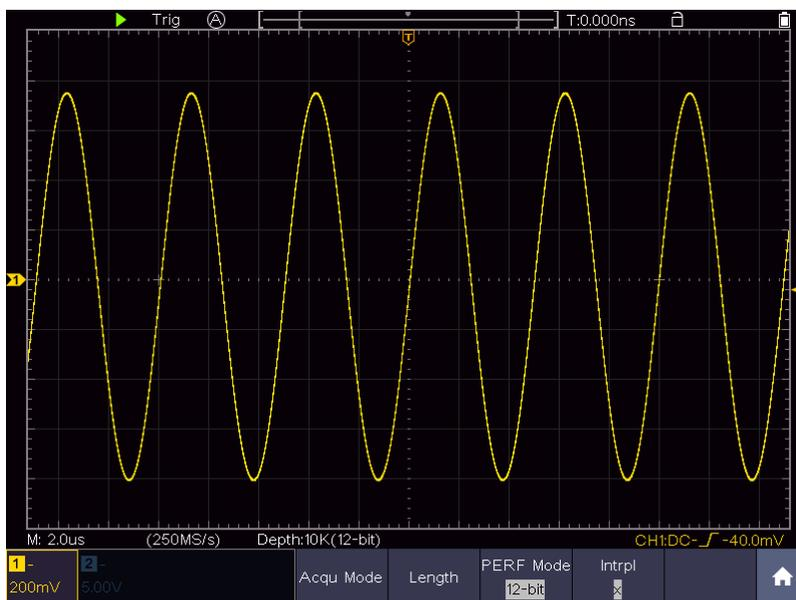
Figure 4-5 Linear interpolation
