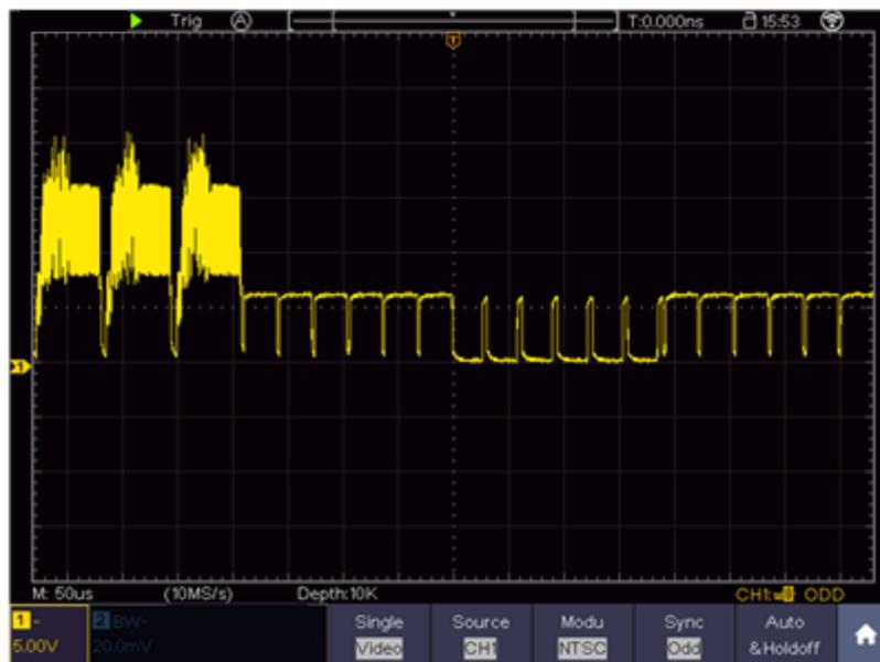
Figure 8-7 Waveform Captured from Video Field Trigger
