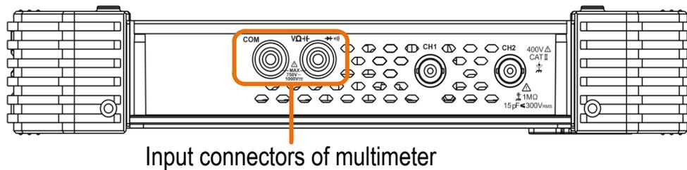
Input connectors of multimeter
