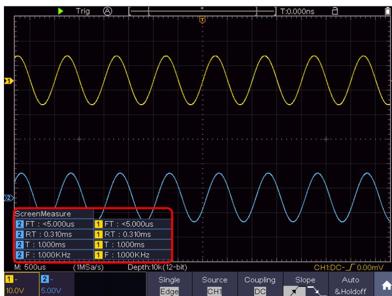
Figure 4-18 Automatic measurement
