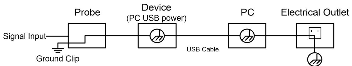
It is NOT allowed to measure AC power when the device been powered by AC power source through the adapter, or when the device powered by PC through USB connection cable (via USB communication interface of PC, with PC powered by AC power source).
