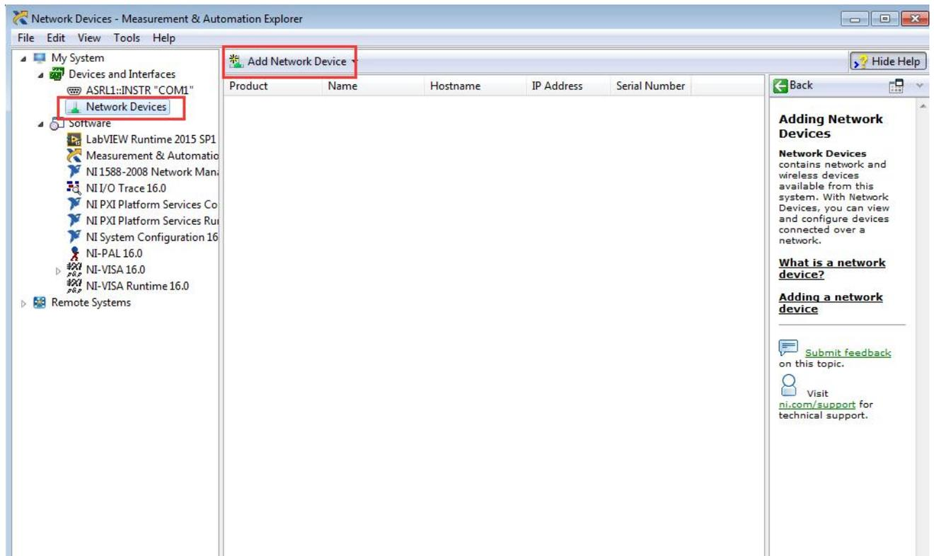
via “Devices and Interfaces”, then “Network Devices”, enter into “Add Network Device”
