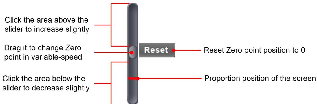
to reset zero point position will change the vertical position of the signal, via moving the slider upwards, or downwards - the farther slider from the center of control bar, the faster the vertical position changes.
