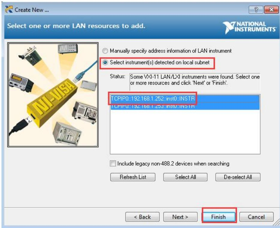
dot-tick "Select instrument(s) detected on local subnet", to choose "TCPIP0::(the previous IP connection just added)::inst0::INSTR", then mouse-click "Finish".
