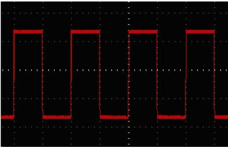
Following illustration is signal output under Peak Detect mode, the interrupting signal noise been captured in details,
