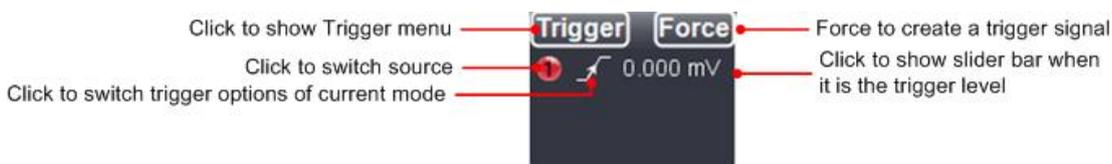
**Force (Trigger):** to create a trigger signal by force, mainly work for "Normal" and "Single" mode under "Trig Mode".
