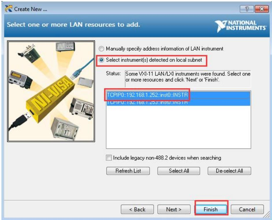
dot-tick “Select instrument(s) detected on local subnet”, to choose “TCPIP0::(the previous IP connection
